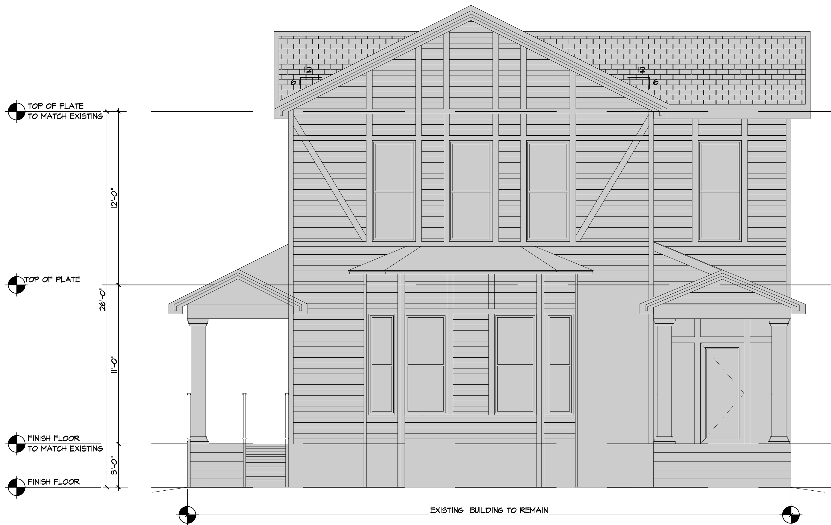
01 new work exterior elevation SCALE: 1/4" = 1'- 0"
